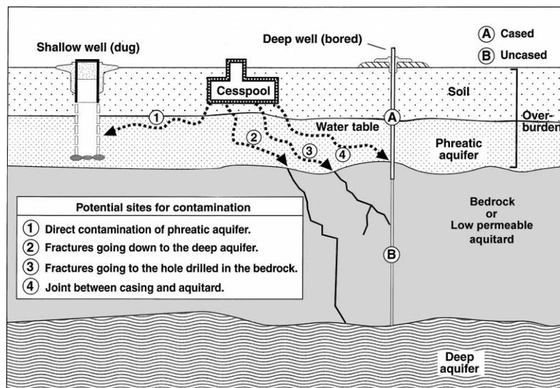
Figure 4. Schema of shallow (dug) and deep (bored) wells and potential sites of HAV contamination
